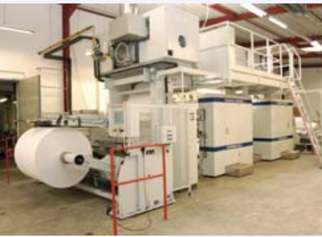
Flexographic press for water-based ink systems
